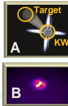
Upon acquiring the LO target, the KW performs divert maneuvers to approach the target. Additional refinement of the intercept calculations are made by the KW and final intercept divert maneuvers are conducted. The KW impacts the target, destroying it with the sheer energy of impact (inset B).
