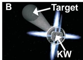
As the IRBM target continues along its trajectory, *O'KANE's* SPY-1 radar detects and acquires the ballistic missile target and associated objects. The Aegis weapon system correlates Aegis SPY tracks with TPY-2 tracks. Based on SPY (local) track data, the weapon system uplinks track information to the missile. With uplink commands, the weapon system positions the SM-3 missile so that the target is in the center of the IR seeker's field of view.
