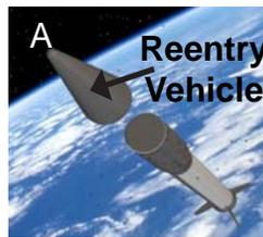
second stage Dual Thrust Rocket Motor separates after motor burnout. Pulse 1 of the Third Stage Rocket Motor (TSRM) fires, providing the axial thrust required to maintain the missile's trajectory. The TSRM's Attitude Control System (ACS) performs a pitch maneuver, ejecting the nosecone and exposing the Kinetic Warhead's (KW) Infra-Red (IR) seeker. The ACS re-aims the missile towards the target. The TSRM executes the Pulse 2 burn.
